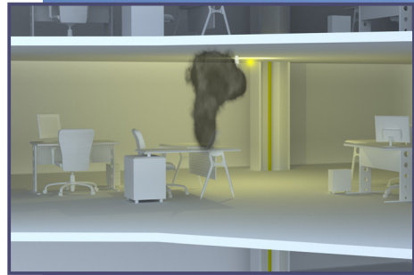
DETECTION THROUGH BURST OF SPRINKLER HEAD
